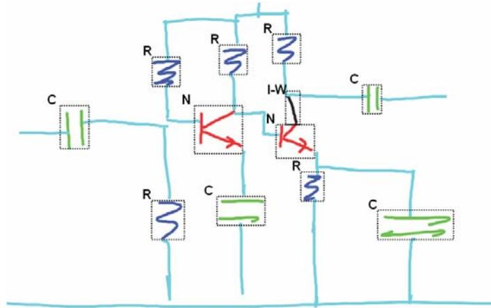
Figure 1: A freehand circuit overlaid with our system's interpretation. The domain has five objects – resistor (R), capacitor (C), npn-transistor (N), wires (W), battery (B). System's interpretation is indicated with colors and labeled boxes. Wires are not annotated to keep the figure uncluttered. This figure also illustrates our system's ability to recognize interspersed drawing – indicated by I-W (see [3] for details).
