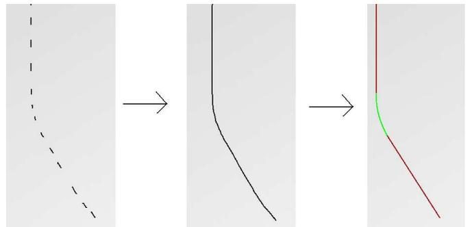
**Figure 2. The three phases of fragmentation.** A continuous curve is obtained by connecting line segments with Bézier curves. Then, the entire stroke is segmented into linear curved segments using its global properties.
