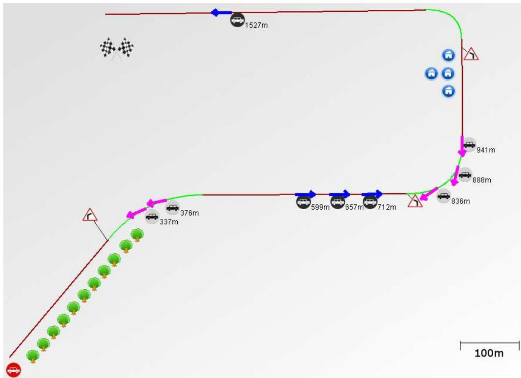
Figure 1. Screenshot of MIRA: Multimodal Intelligent Road Design Assistant. The road is displayed as a series of straight and curved segments. The vehicle icon in the lower left corner indicates the starting point of the drive in the simulator. Vehicles making up the traffic are annotated with their direction of travel, and distance from the start line of the simulation. Other elements of the road design include the trees, buildings, and signs.
